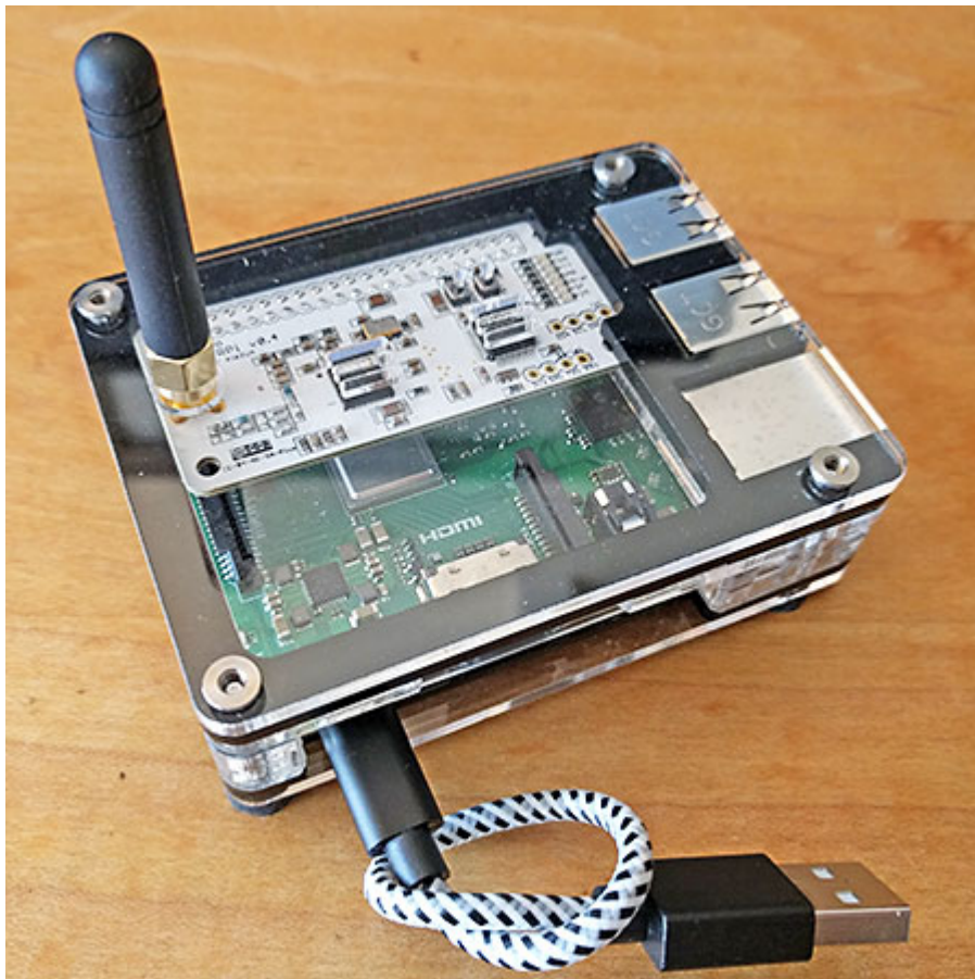
C4Labs case for a simplex hotspot with the RPi 3B/3B+ form factor
