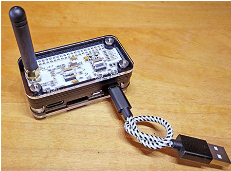
C4Labs case for a simplex hotspot with the RPi Zero W/Zero 2 W form factor
